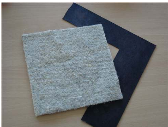
Fig. 3 Example of hemp non-woven mat and of the high resin composite produced by impregnating it with a tannin-based resin
