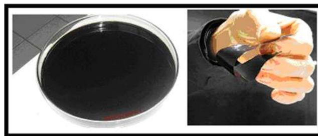
Fig. 4 Flexible tannin/furanic films and surface finishes
