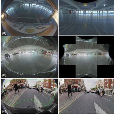
Figure 4: Undistorting the fisheye image: (a) Rectilinear correction; (b) Piecewise linear correction; (c) Cylindrical correction. Left: raw image; Right: undistorted image.
