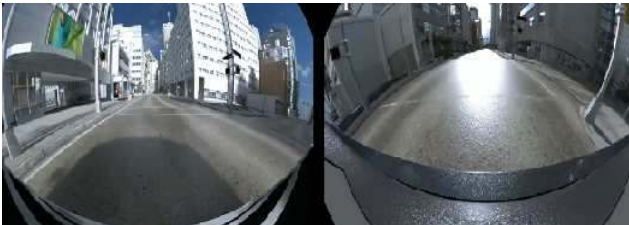
Figure 10: Synthetic images modelling fisheye optics
