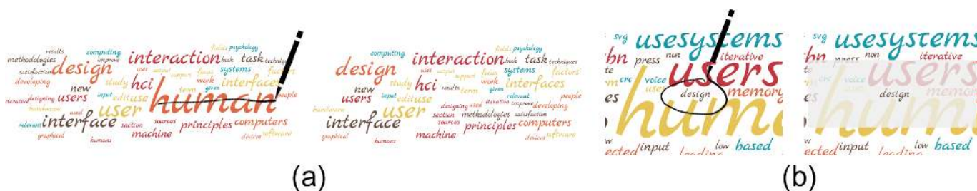
Figure 4: Pen interaction. (a) People can strike through a word to remove it; after the word disappears, words that are located at the boundary of the wordle move to fill the blank area. (b) People can draw a circle that encompasses the word to select a word too small to be selected with a touch; upon selection, a handle for manipulation appears.
