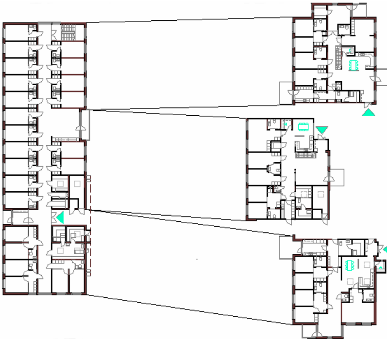
Fig. 58. Architectural plan of the restructuring of the old wings of City Home into small units (reproduced from Riippa 1998).
