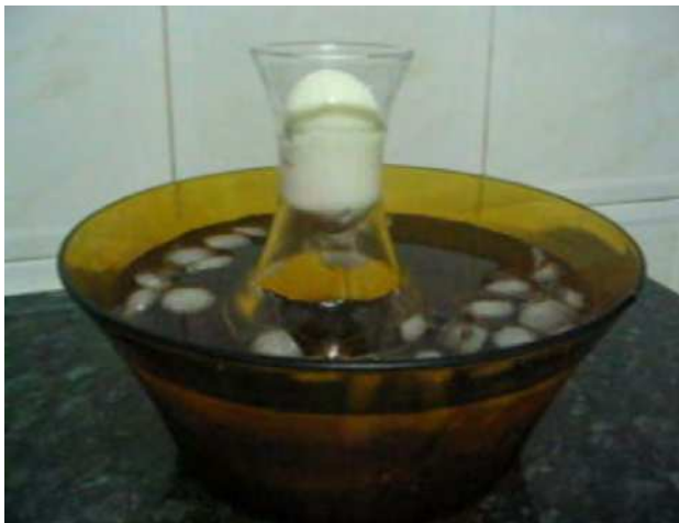
Fig. 2. Egg moving downwards by pressure difference
