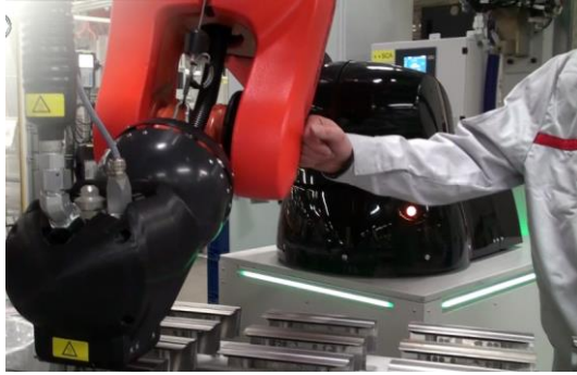
Fig. 7: MRK-Systeme robot during the gluing process. The safety skin of the robot detects human contacts. The end-effector is framed by a plastic case.
