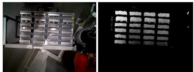
Fig. 6: Camera view (left) and segmented depth image (right) of the glued reinforcement plates. White pixels represent near points and dark pixels represent distant point.
