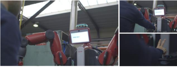
Fig. 2: Proof of concept using the Baxter robot for multimodal interactions (gestures and face recognition).
