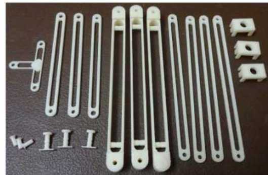
Fig. 6 RPT 3D part models printed using Stratasys FDM 360mc
