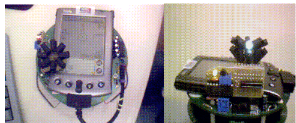
Figure 4. The Augmented Reality Mast (ARM) projects information from the robots to a user's head-mounted display.
