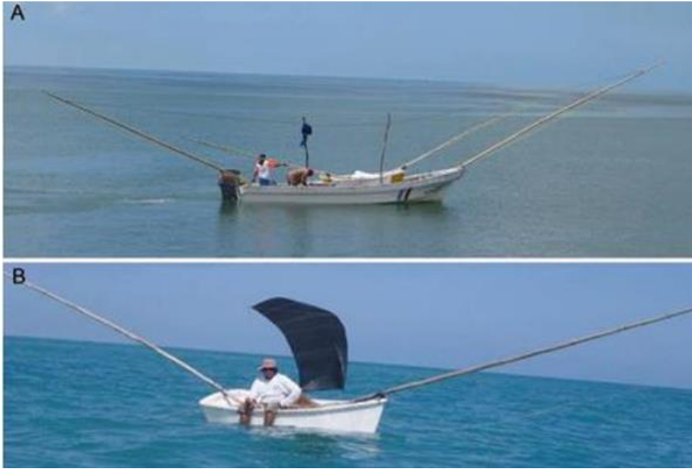
Figure 9. Al garete fishing style used for the Octopus maya fishery. A, a motor boat with fishing lines carrying inside a small boat called "alijo". B, the "alijo" with the small sail called "garete" extended, used to derive taking advantage of the wind. From Markaida et al. (2015).
