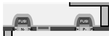
Fig. 5: TFT utilizes majority carrier accumulation devices due to drive current enhancement.
