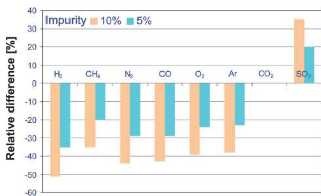
Fig. 5 Effect of impurities on the storage density in comparison to pure CO 2 (120 bar).
