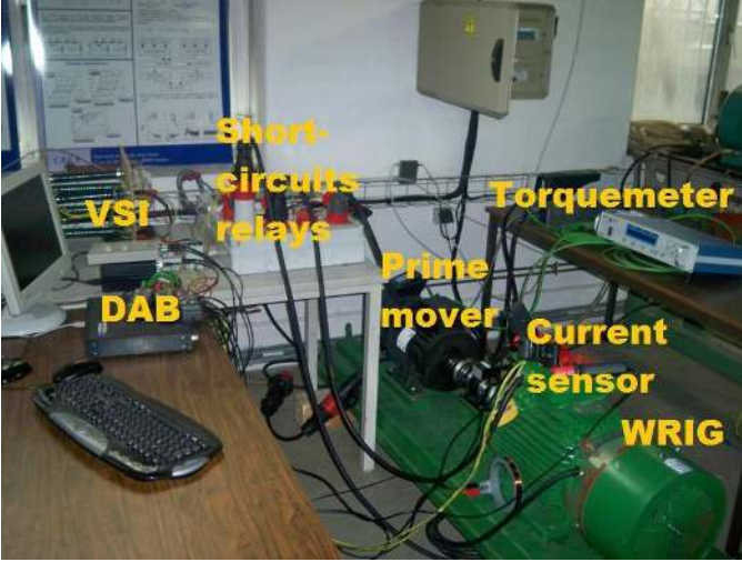
Fig. 4. Set-up for the different tests: a) Block-scheme configuration b) Photo of the real set-up.
