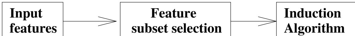
Figure 4.2: The feature filter approach, in which the features are filtered independently of the induction algorithm.
