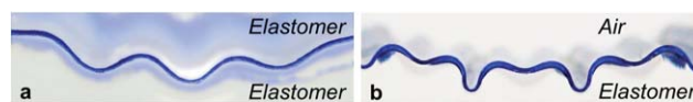
Fig. 8 Comparison between profiles of a compressed membrane resting in between two identical soft PDMS foundations (trilayer, a) and a compressed membrane bound to a soft PDMS foundation (bilayer, b) for a similar relative compression \delta \approx 0.23 .
