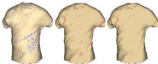
Figure 6: Deformation: (left) anchor triangles (fold edges projected to input garment); (center) vertex positioning result; (right) garment after stretch reduction. The coloring (center, right) shows per-triangle stretch. The iterations reduce the maximal per-triangle stretch from 8% to 4%.
