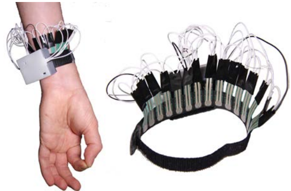
Figure 1: WristFlex prototype. Left image: device worn on the wrist, while performing a finger pinch gesture. Right image: the side of the device that contacts the skin, exposing an array of force sensitive resistors (FSRs).
