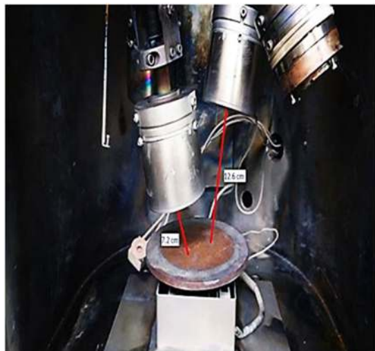
Figure 2. Physical view of the pinhole reduction technique.
