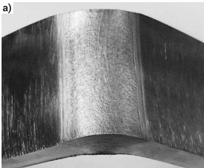
Rys. 6. Widok spoin po próbie gięcia: a) lico spoiny, b) grań spoiny Fig. 6. View of joint after bending test: a) face side, b) root side
