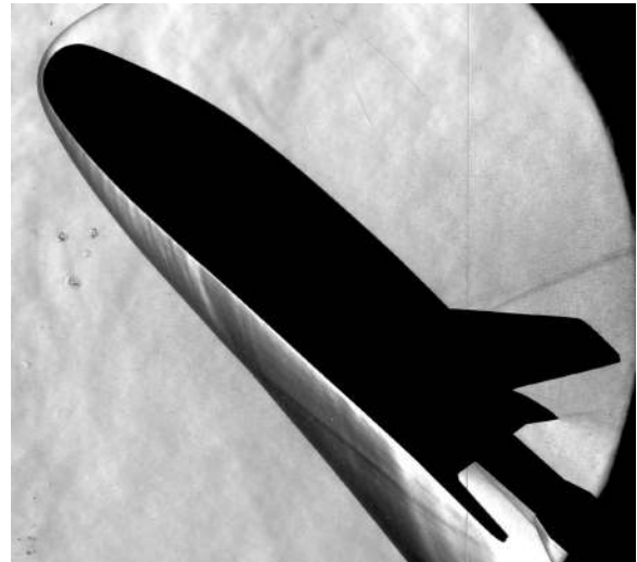
Fig 22 Effect of k=0.008-in extended bowed panels on bow shock for \alpha = 40\text{-deg} , Re = 4 \times 10^6/\text{ft} , \delta_{BF} = 0\text{-deg}
