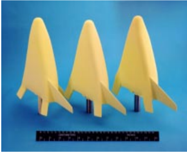
Figure 5 Photograph of X-33 Rev-F models with various flap deflections.
