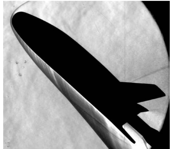
Fig 22 Effect of k=0.008 -in extended bowed panels on bow shock for \alpha = 40 -deg, Re = 4 \times 10^6 /ft, \delta_{BF} = 0 -deg
