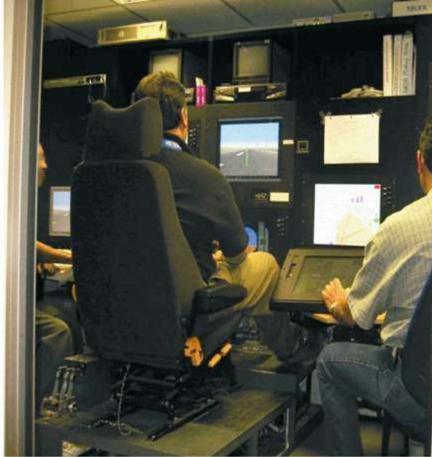
Figure 4. The ground control station in use. The pilot (center) uses both the head-up display, providing a view out the aircraft nose, plus key aircraft performance indicators along with the lower head-down display. The test engineer, on the right, interacts with the aircraft through the touchscreen display panel. The Range Safety Officer, just visible on the left, ensures that the aircraft remains safely inside the range boundary.
