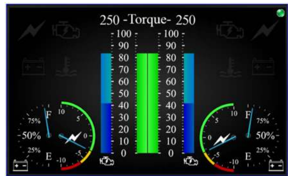
Fig. 9. The X-57 cockpit display reflects the duality of the X-57 system design. Indicators include State of Charge, discharge rate, and throttle position.
