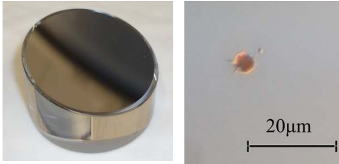
Figure 1: The multilayer-coated off-axis parabola (left) and an optical differential interference micrograph of a single-shot crater created near the focal plane (right).
