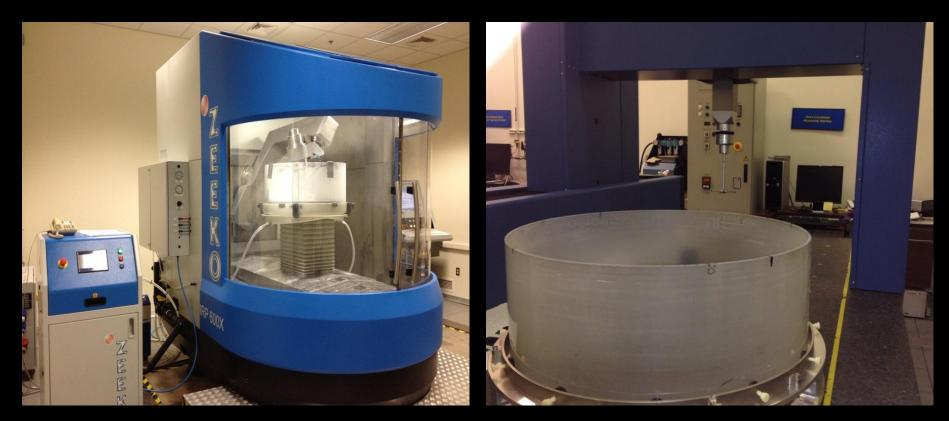
Research in direct fabrication of thin-walled full-cylinder grazingincidence optics utilizes a freeform robotic polisher. Precision measurements with metrology instruments—including a Coordinate Measuring Machine are essential during fabrication.
