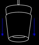
Separate the shell from the mandrel in a cold-water bath; clean mandrel for additional replications.
