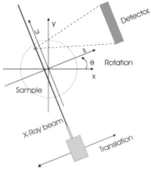
Figure 3: Diagram of fluorescence tomography [5].
