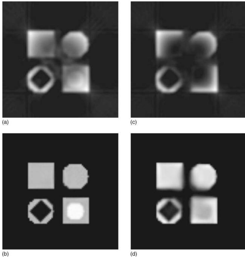
Figure 2: Simulated iron and calcium distributions. (a) Iron without correction for attenuation. (b) Iron with correction for attenuation. (c) Calcium without correction for attenuation. (d) Calcium with correction for attenuation. [1]
