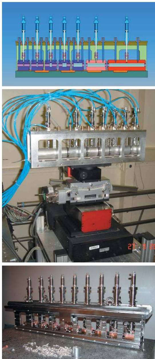
Figure 1 Schematic illustrating the transfocator concept (top), the IAT installed on the beamline (middle) and the IVT during assembly (bottom).
