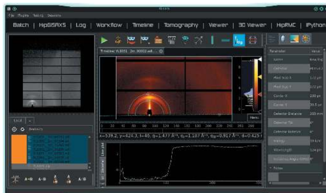
Figure 2 A 300 frame data series from an OPV drying experiment loaded in Timeline. The crystalline peak arc has been selected on the image (cyan). The reduced data displayed in the bottom panel show the integrated intensity in the selected region. This shows that crystallization began around frame 100; however, dynamics continue to drive structural change to a lesser degree, as indicated by a drop in intensity towards frame 250.
