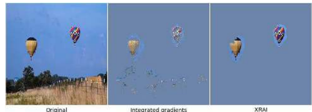
Figure 1. Comparison of Integrated Gradients (middle) and the proposed XRAI method (right) at 5% area threshold for object class “balloon”. Areas that may have high pixel-level attributions are removed at the region level as they sum up close to zero.
