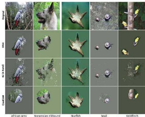
Figure 8. XRAI (2nd row) compared to Integrated Gradients with random baselines (3rd row) and GradCam (bottom row). Grad-Cam can produce blobby regions, whereas XRAI tend to create regions tightly bound around identified objects.
