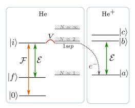
FIG. 1. Schematic representation of the level scheme. A helium atom in the ground state 0 is resonantly photoexcited to the selected doubly excited state i, which is coupled to the continuum and decays via fluorescence to a singly excited state f or via autoionization a to  $He^+$  1s. The latter is coupled to  $He^+$  2p (b) by the emitted radiation.
