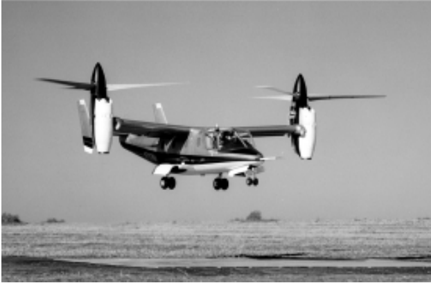
Figure 1. XV-15 tiltrotor aircraft hovering over hover pad at the test site near Waxahachie, Texas.
