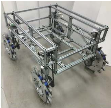
L1100mm×W850mm×H580mm, 68kg Wheel base (620~)780mm DC motor 63W×4, Gear ratio 6192:1
