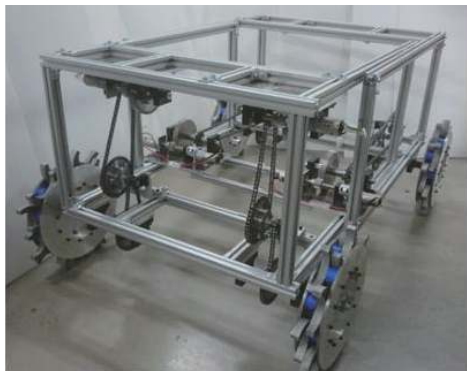
L1300~1650mm×W1000mm×H830mm, 85kg Wheel base 930~1280mm DC motor 63W×4, Gear ratio 8357:1
