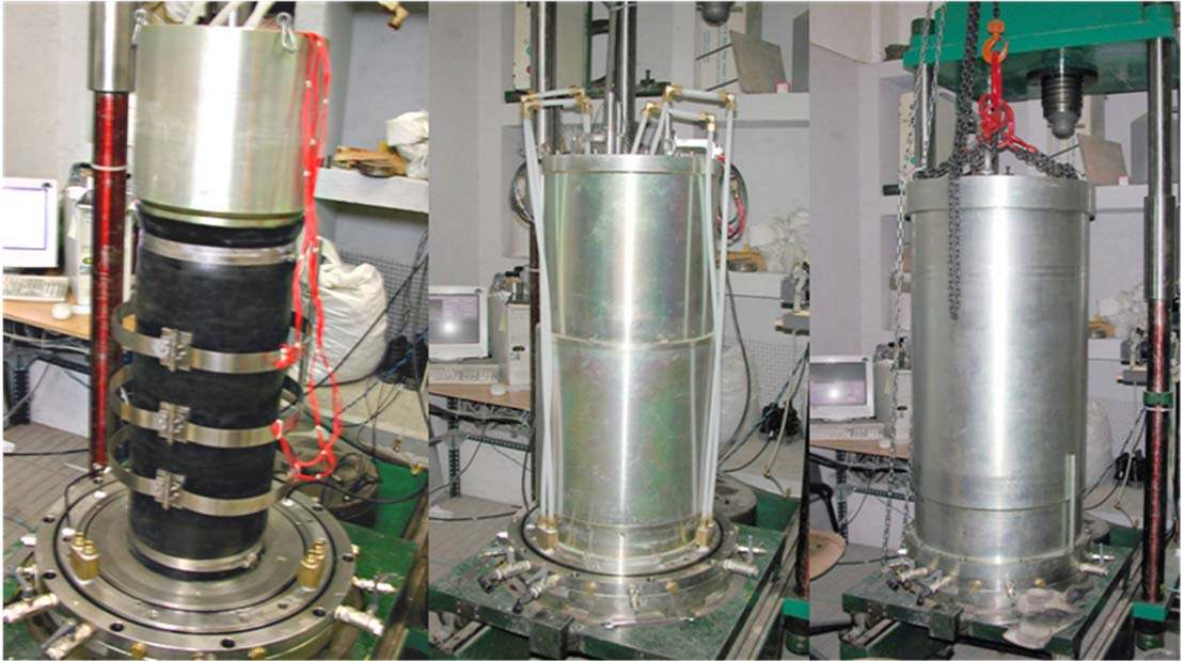
Figure 4: a) Triaxial sample after installation of sensors for volume change; b) Placement of inner cell wall; c) Installation of outer cell wall.
