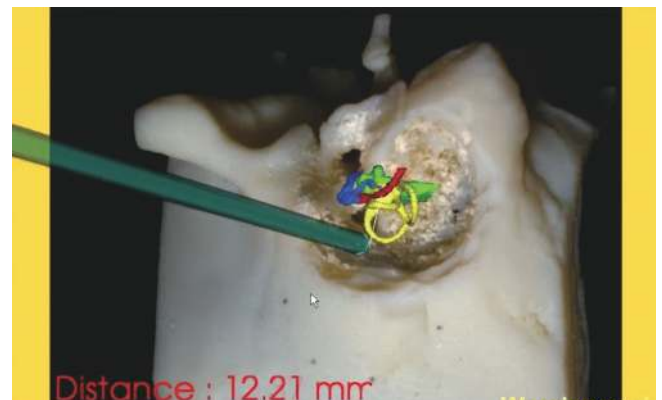
Fig. 4. Depth information is provided in quantity at lower left corner, and background color (yellow) shows the level of potential risk.
