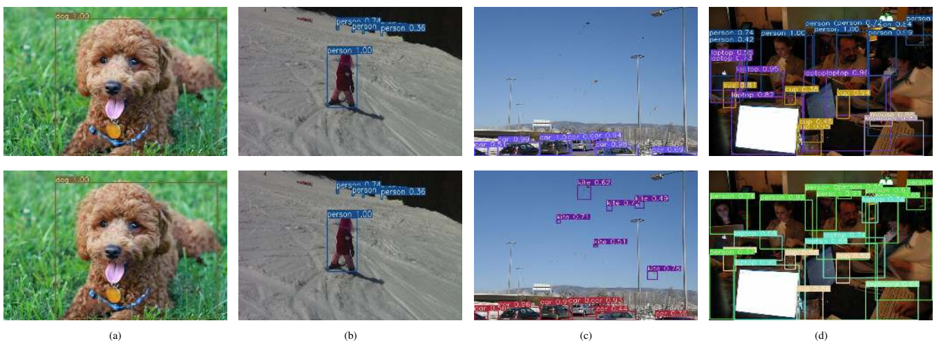
FIGURE 9. Comparison of the detection results of YOLOv3 (the top row) and YOLO-ACN (the bottom row) on typical images on the test set of MS COCO 2017. The detection result of the large size object in the (a) are similar, and the small objects can also be detected well with the proposed YOLO-ACN network, e.g., the long-distance person in (b); the kites and cars in (c); the cups and laptops in (d).
