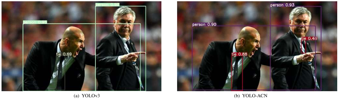
FIGURE 10. Comparison results of object occlusion problem. (a) the detection result of the YOLOv3, (b) the detection result of the YOLO-ACN. The tie which occluded by the arm can be detected with the proposed YOLO-ACN network, whereas the YOLOv3 cannot detect it.
