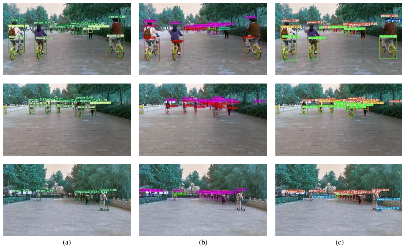
FIGURE 13. Video detection results of some typical frames. (a) Results of YOLOv3. (b) Results of YOLOv4. (c) Results of YOLO-ACN. Compared with YOLOv3 and YOLOv4, YOLO-ACN has an amazing performance on small targets and occluded objects detection, for example, the cell phone in the first image of the column (c), the person beside the tree in the second image, and the skateboard in the third image.
