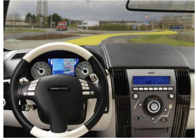
Fig. 5. AR navigation system with head-up display from Siemens-VDO 2005.
