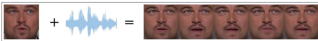
Fig. 1 The Speech2Vid model generates a video of a talking face, given still images of the person and a speech segment. In the output video the talking face is lip synched with the audio. Note, only one input
