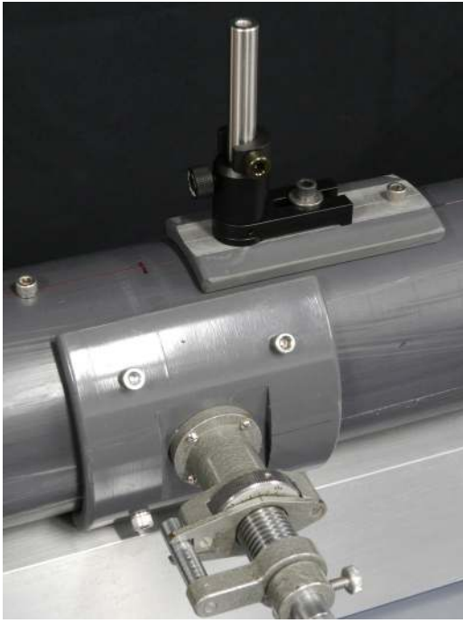
Fig. 4. Both the marker and eraser assemblies attached to the PVC pipe. The eraser polarizer is moved into place by simply lowering the lens post. No fine adjustments are necessary.
