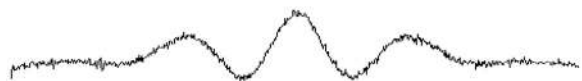
Fig. 11. Double-slit interference with an incandescent light source. The graph and image grayscale is 0–1000 counts.
