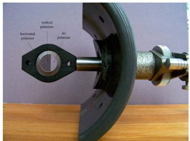
Fig. 3. The which-path marker (left) consists of vertical and horizontal polarizers held by a standard lens mount; its position is adjusted from outside the PVC pipe.
