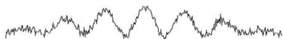
Fig. 10. With the quantum eraser in place, the double-slit interference is restored. The graph and image grayscale is 0–1000 counts.
