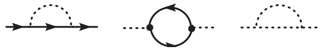
FIG. 2. Self-energies for scalar and fermion fields induced by the Yukawa and triscalar interaction Lagrangians of Eqs. (15) and (20).
