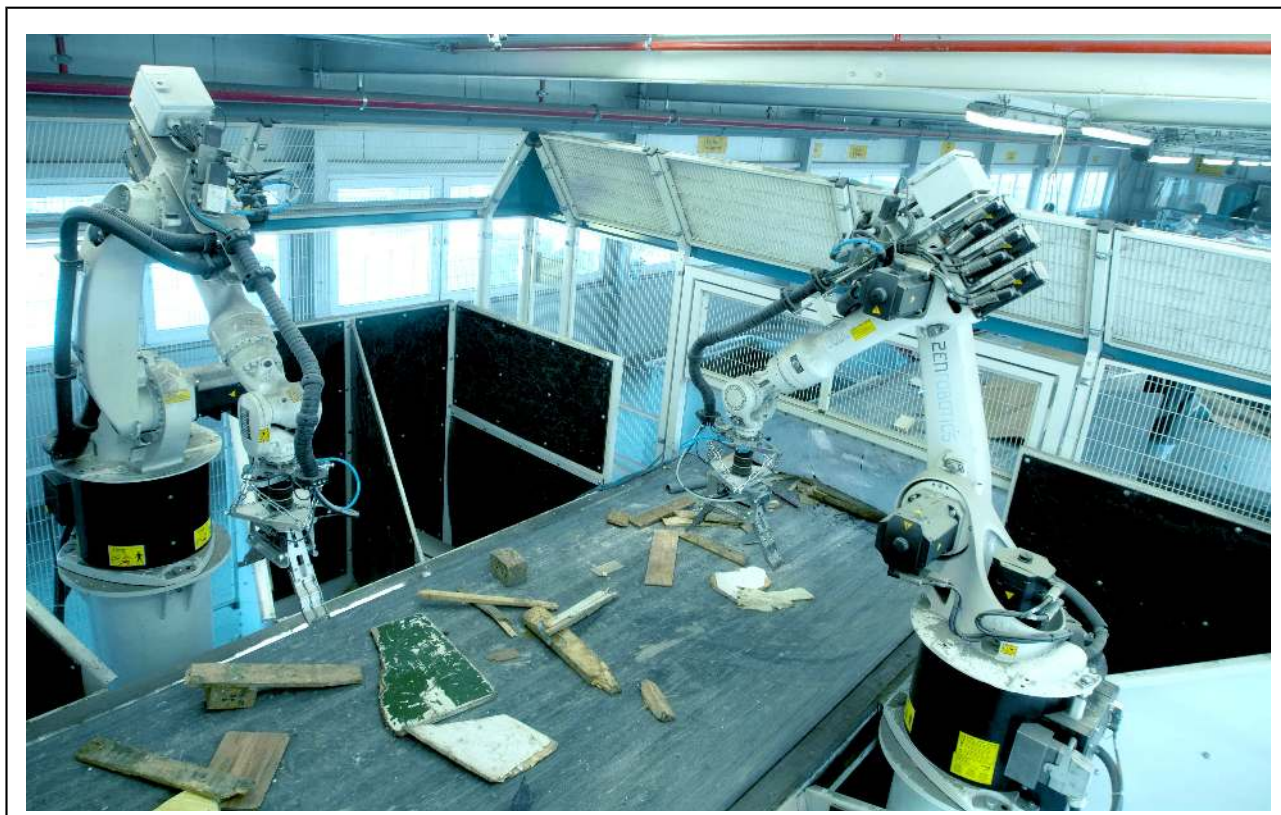
Figure 4: Retrofit ZRR Fast Picker system installation. (Image © ZenRobotics Ltd 2014. Used with permission.)
