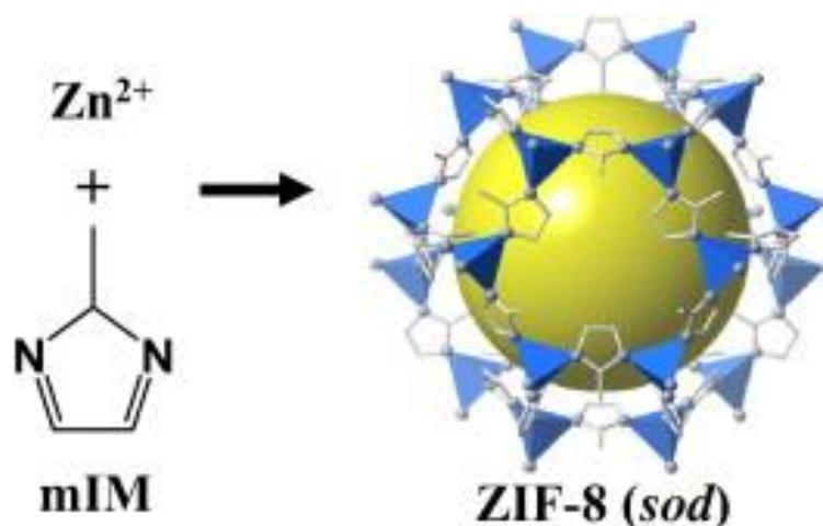
Crystal structure of ZIF-8: Zn (polyhedral), N (sphere), and C (line)
