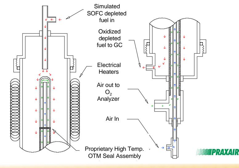
Fabricate OTMs and test in SOFC depleted fuel - Short tubes
