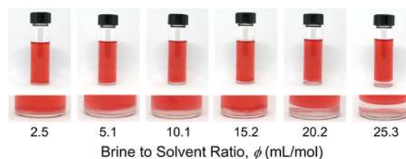
Figure 3. Photographic images of 5.0\ \text{M} NaCl brine combined with DIPA solvent at brine volume to solvent mole ratios, \phi , of 2.5 , 5.1 , 10.1 , 15.2 , 20.2 , and 25.3\ \text{mL/mol} . For better visualization of the two phases (i.e., solvent and aqueous layers), oil red O dye was dosed to stain the solvent. Only two phases (solvent and solid) were observed for \phi of 2.5 – 15.2\ \text{mL/mol} , whereas an additional aqueous phase was noticed for \phi of 20.2 and 25.3\ \text{mL/mol} .
