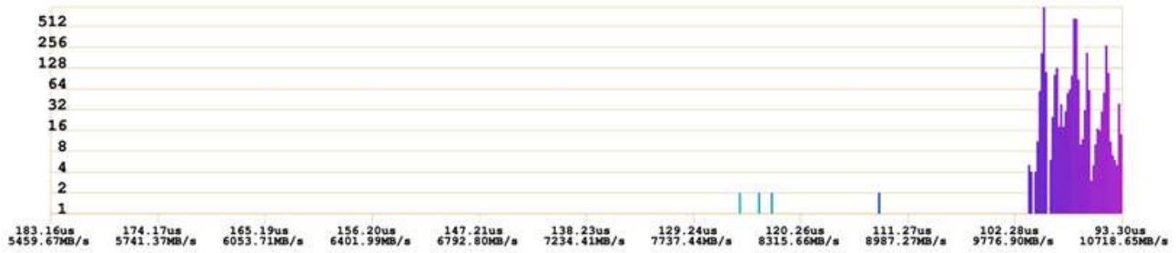
Figure 5: Histogram of the ping-ping times/speeds between all nodes using 1 MB packets in serial mode
