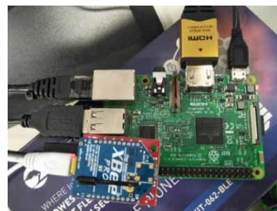
Fig. 12. Raspberry Pi 3 and Zigbee RF Module Connectivity.
