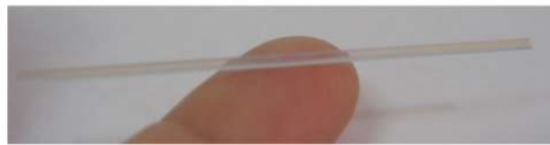
Fig. 3. (Color online) (a) Two-dimensional view of the slab with dimensions and coating properties. (b) Photograph of a fabricated Nd:YAG slab.
