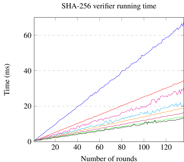
Figure 8: Relation between the total running time and the number of rounds for the SHA-256 verifier, average over 100 runs.
