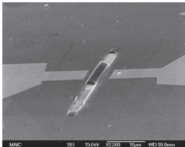
Fig. 3. Scanning electron microscopy of ZnO nanorod with integrated microchannel (4- \mu\text{m} width).
