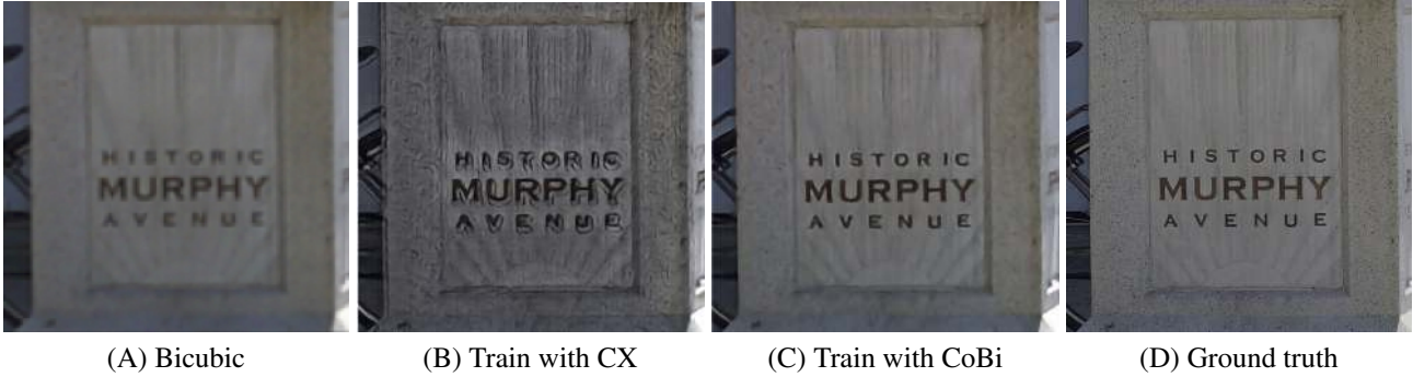
Figure 3: Training with the contextual loss (CX) results in periodic artifacts as shown on the flat wall in (B). These artifacts are caused by inappropriate feature matching between source and target images, which does not take spatial location into account. In contrast, training with the proposed contextual bilateral loss (CoBi) leads to cleaner and better results, as shown in (C).
