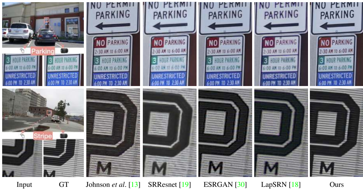
Figure 5: Our 4x zoom results show better perceptual performance in super-resolving distant objects against baseline methods that are trained under a synthetic setting and applied to processed RGB images.
